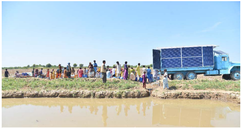
Our solar-powered mobile reverse osmosis plant converts contaminated flood water into water that is safe for drinking.
